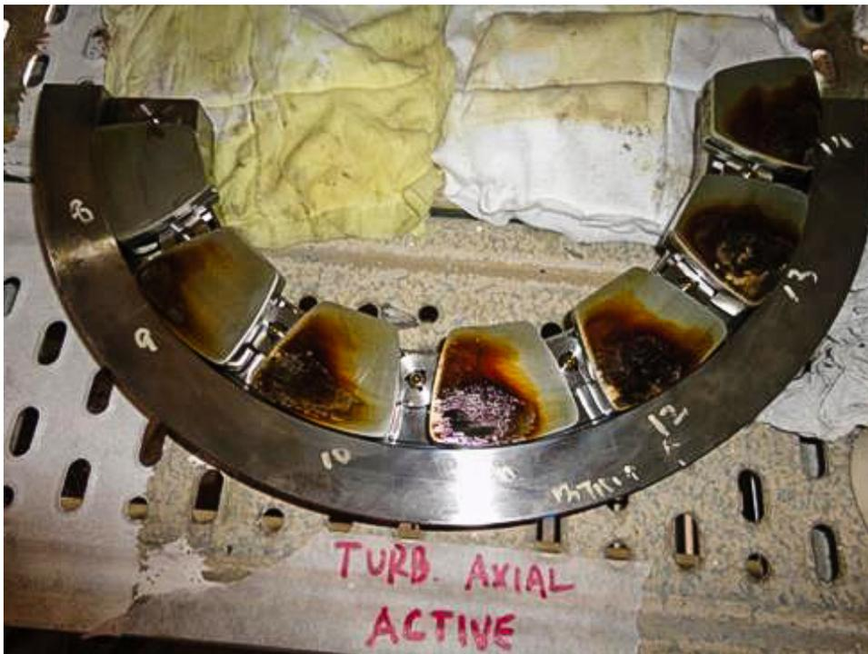
*Figure 5: Deposit formation on a bearing, showing surface damage at its highest load zone.*
