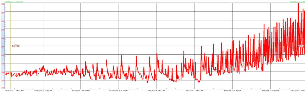
**Figure 1: Bearing temperature increase in a compressor**
