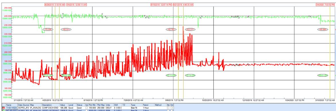
**Figure 9: The impact of adding Solvancer(tm) technology to an compressor's bearing temperature.**
