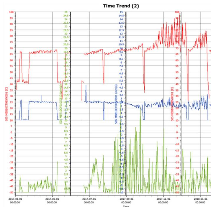
**Figure 2: Increases in axial bearing temperatures (red) are correlated to increases in vibration signals (green)**
