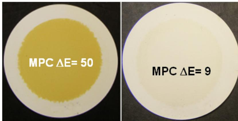
**Figure 8: Example Patches and values from the Membrane Patch Colorimetry (MPC) test. A value of 50 would be considered critical, warranting immediate action. A result of 9 would be considered acceptable.**
