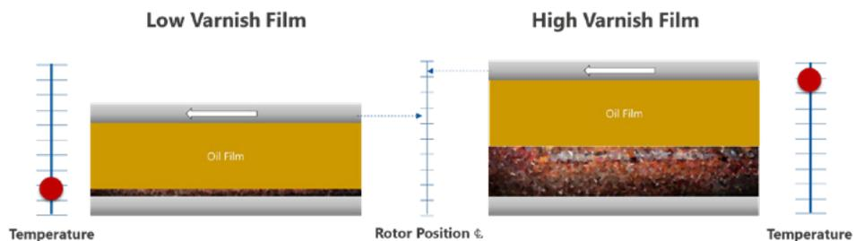
**Figure 4: Illustration suggesting the impact that varnish deposits have on bearing temperatures and rotor position.**
