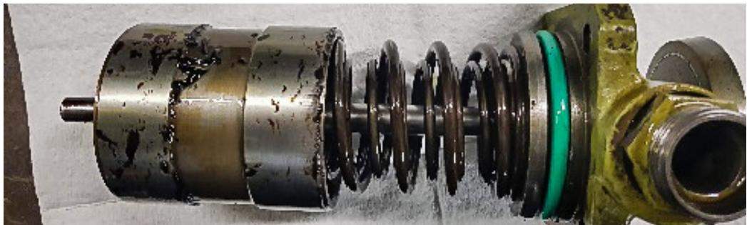
*Figure 6: A Failed valve coated with varnish deposits.*
